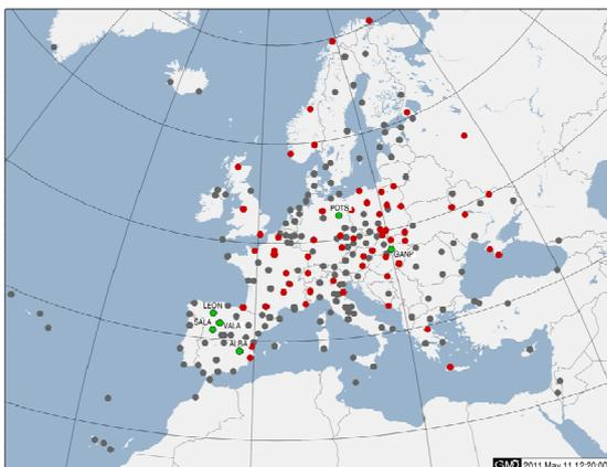
**Fig. 3:** Map of EPN with GNSS equipment capable of tracking L5. Stations in green include the L5 signal in their RINEX observation files; stations in red do not.
