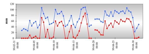
Fig. 10 Zenith Wet Delay from radiosonde (high) and GPS (BOGO - CODE sloution) (low).
