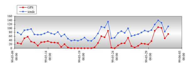
Fig.9 Zenith Wet Delay from radiosonde and WUT solution for JOZE
