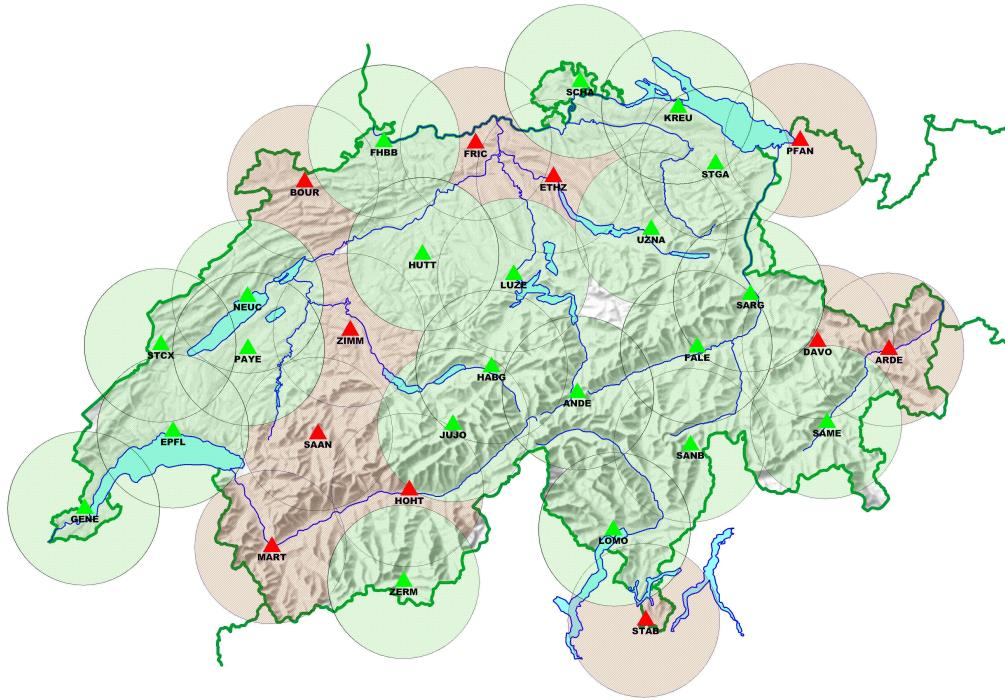
Figure 6: The AGNES network after the transition to combined GPS/GLONASS service: For ten "double sites" (marked in red), the old and new equipment will be run in parallel (PFAN is operated by the Austrian BEV).
