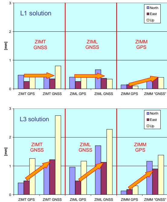
Figure 3: Repeatability values of a L1 solution (top) and a L3 solution (bottom) with fixed ambiguities for GPS-only and combined GPS/GLONASS observations.
