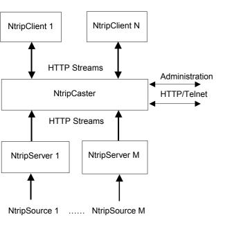
Fig. 1: Ntrip Streaming System
