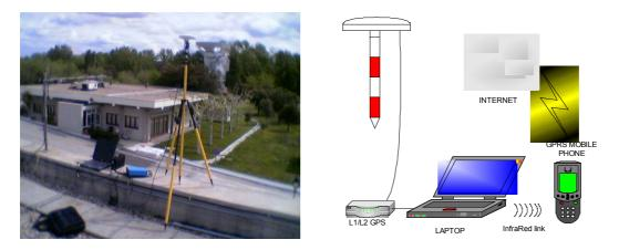
Figure 3: Bench mark Villafranca, 20 km distance from Madrid reference station (left), and General diagram of GPS rover configuration (right)
